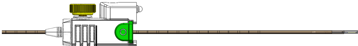
Figure 1.6: NB3 Laser Probe Locking Interface and Floating Depth Stop
