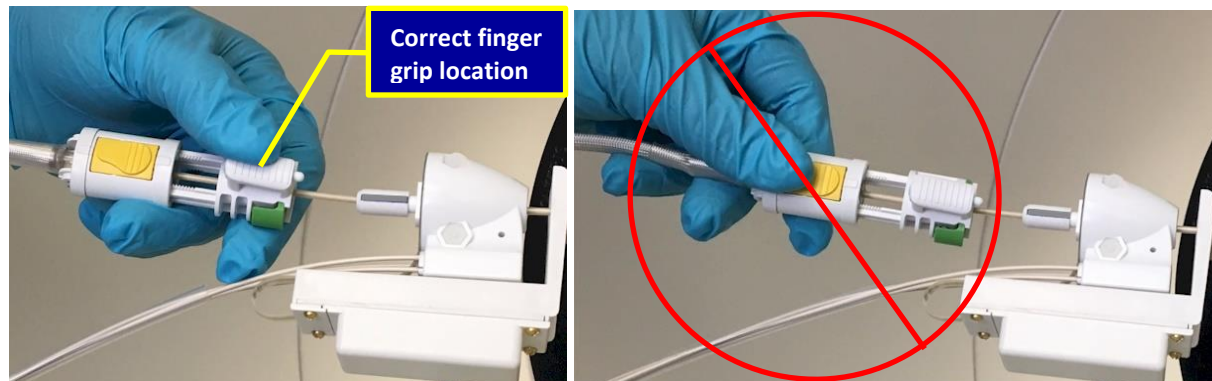
Figure 8.6.42: Left: Correct LDP Insertion Technique; Right: Incorrect LDP Insertion Technique
